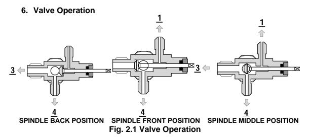
**Back Position**: Process and manometer port closed for normal operation
